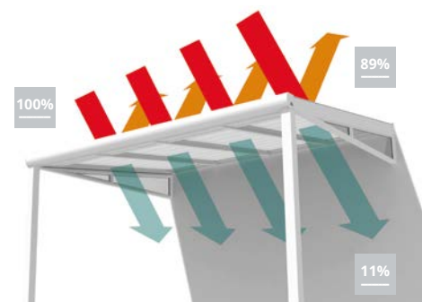
Reflection of heat radiation: Gumax® sun shading
